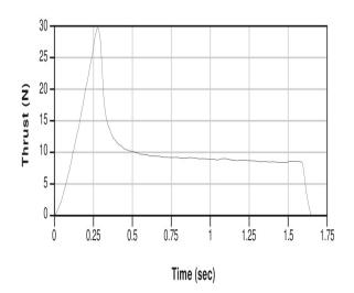
This chart shows the amount of thrust being developed by the motor through the entire burn time (the delay and ejection charge are typically not included in these charts as they do not effect the thrust being developed). A typical motor has a high peak spike thrust during the initial firing of the motor, then drops and levels off, and finally fades out as the last of the propellant is used up. The NAR thrust curve chart on the previous page shows the D12 used in our Goblin example.
